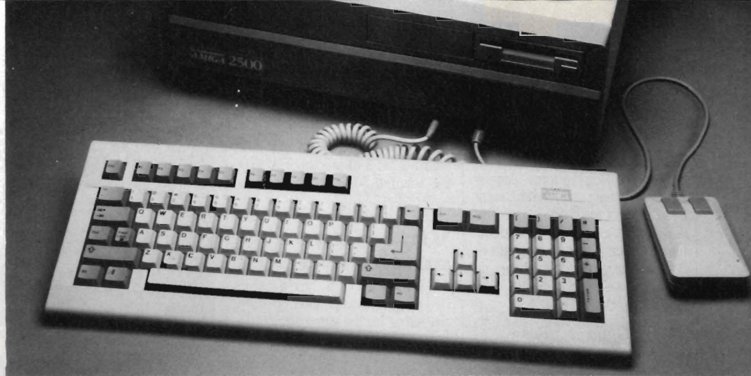
■ The Amiga 2500 – 68020, 2Mb RAM, 68881 maths co-processor. A power user's machine at $4699.
