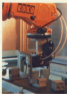
The addition of colour and tactile sensors to a programmable robot arm would be of enormous benefit to industry. This project uses vision systems from Japan's Lead Limited of Tsuzi & Murai to select randomly placed machine parts and put them in a specified position and orientation.
