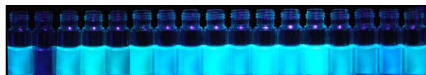
Figure 5. Visual fluorescence changes of 7 (10.0 \mu\text{M} ) upon addition of various metal ions in \text{CH}_3\text{CN}/\text{CHCl}_3 (40:1, v/v). From left to right: free 7 , \text{Cu}^{2+} , \text{K}^+ , \text{Li}^+ , \text{Na}^+ , \text{Cs}^+ , \text{Rb}^+ , \text{Ag}^+ , \text{Co}^{2+} , \text{Ba}^{2+} , \text{Pb}^{2+} , \text{Ca}^{2+} , \text{Hg}^{2+} , \text{Mg}^{2+} , \text{Sr}^{2+} , \text{Zn}^{2+} , and \text{Al}^{3+} (100.0 equiv, respectively).
