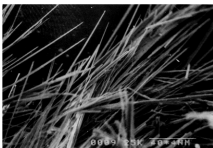
Figure 5. SEM image of peptide 1 showing a bunch of rod-like fibrils in the solid state.
