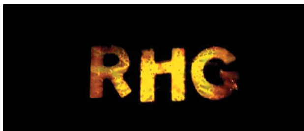
Figure 5. Thin film of 8 irradiated through an RHG mask at 315 nm. Irradiated areas are non-fluorescent.
