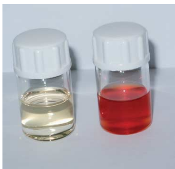
Figure 7. Photograph of two dichloromethane solutions (3 ml) of 1a-PS (50 mg in the first run) that has to be submitted to 10 consecutive test-recovery cycles. Left: upon addition of 500 \mu\text{l} of an 2.5 \times 10^{-3} M ethanolic solution of \text{Mg}(\text{OAc})_2 . Right: after addition of 50 \mu\text{l} of an 2.5 \times 10^{-3} M solution of \text{Fe}(\text{NO}_3)_3 .
