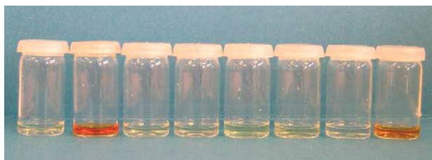
Figure 2. Colour changes observed in \text{CH}_3\text{CN} solutions ( 1 \times 10^{-2} M). From left to right (a) free ligand 1 , (b) 1 + \text{F}^- , (c) 1 + \text{Cl}^- , (d) 1 + \text{Br}^- , (e) 1 + \text{I}^- , (f) 1 + \text{HSO}_4^- , (g) 1 + \text{H}_2\text{PO}_4^- , (h) 1 + \text{F}^- + \text{Cl}^- + \text{Br}^- + \text{I}^- (10 equiv of tetrabutylammonium salts for each anion were used).
