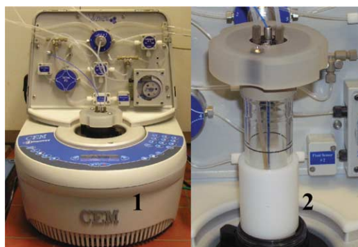
Figure 1. Voyager platform (1) and 80 mL glass vessel (2).
