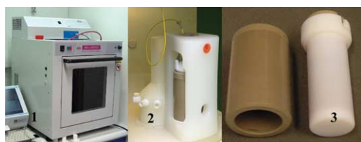
Figure 3. MicroSYNTH platform (1), control vessel rotor segment (2), high-pressure sleeve, insert and cap of a standard vessel assembly (3).
