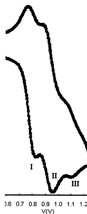
Figure 7. CVs of a 10 −3 mM 4 solution in 0.10 M Bu 4 NPF 6 /MeCN. Potential scan rate 100 mV/s.
