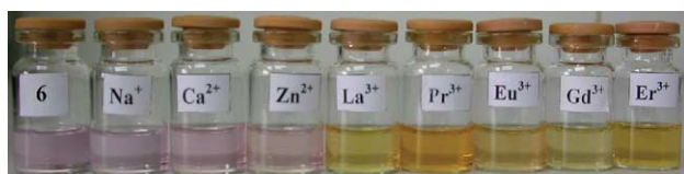
Figure 1. Color change of compound 6 (50 \mu\text{M} ) in acetonitrile induced by addition of 2 equiv of metal nitrate (from left to right: compound 6 without metal ion; addition of \text{Na}^+ ; \text{Ca}^{2+} ; \text{Zn}^{2+} ; \text{La}^{3+} ; \text{Pr}^{3+} ; \text{Eu}^{3+} ; \text{Gd}^{3+} ; \text{Er}^{3+} ).
