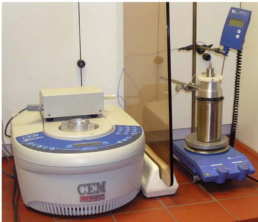
Figure 3. Experimental setup for the determination of a heating profile (via the microwave software) of an experiment executed in an oil bath.
