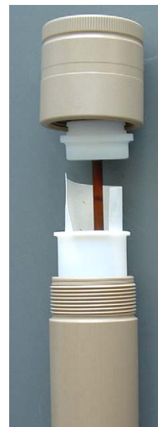
Figure 2. Reaction format for MW-assisted macroarray reactions. Shown is a macroarray that was rolled and placed into a 70 mL Milestone Teflon/PEEK reaction vessel. Reactions are performed in reusable Teflon inserts (white) that fit inside the PEEK outer casing (beige). A ceramic sheath in the center (brown) houses a fiber-optic probe for direct temperature measurement during the reaction. Vessel dimensions: 12 cm tall with an internal diameter of 3 cm.
