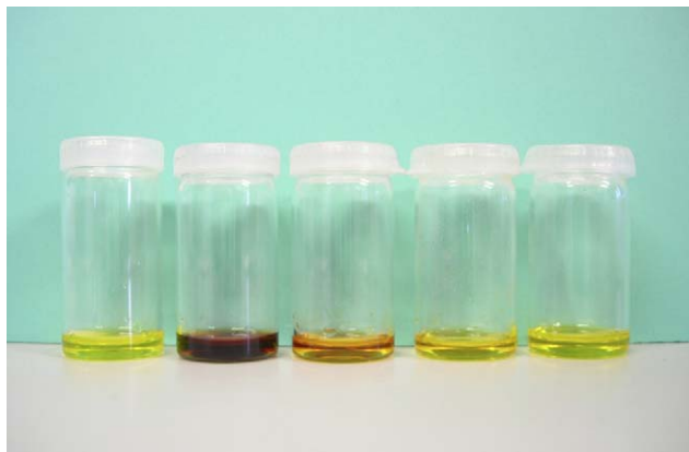
Figure 4. Colour changes observed on addition of TBA salts (10 equiv) to a DMSO solution of receptor 3. Left to right: no addition, fluoride, acetate, o -methoxybenzoate and o -nitrobenzoate.
