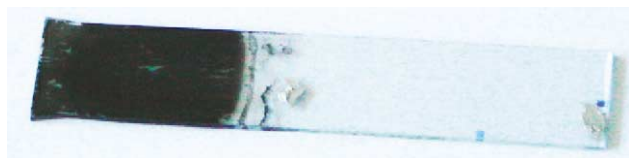
Figure 11. PTPC polymer films electrochemically deposited on ITO glass after electrical measurements.
