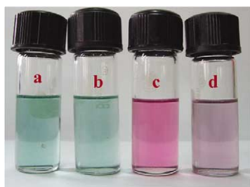
Figure 7. Colour of dichloromethane solutions of \text{USqH}^+ ( 15 \mu\text{M} ) (a) in the absence of metal ions, (b) in the presence of 0.3 \text{ mM Li}^+ , \text{Na}^+ , \text{Mg}^{2+} , \text{Ca}^{2+} , \text{Ba}^{2+} , \text{Zn}^{2+} and 100 \mu\text{M Cu}^{2+} (c) in the presence of 40 \mu\text{M Hg}^{2+} and (d) in the presence of 87 \mu\text{M Pb}^{2+} .
