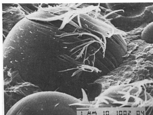
Fig. 9. Fracture surface of a PBT/Vectra (65:35) blend.
