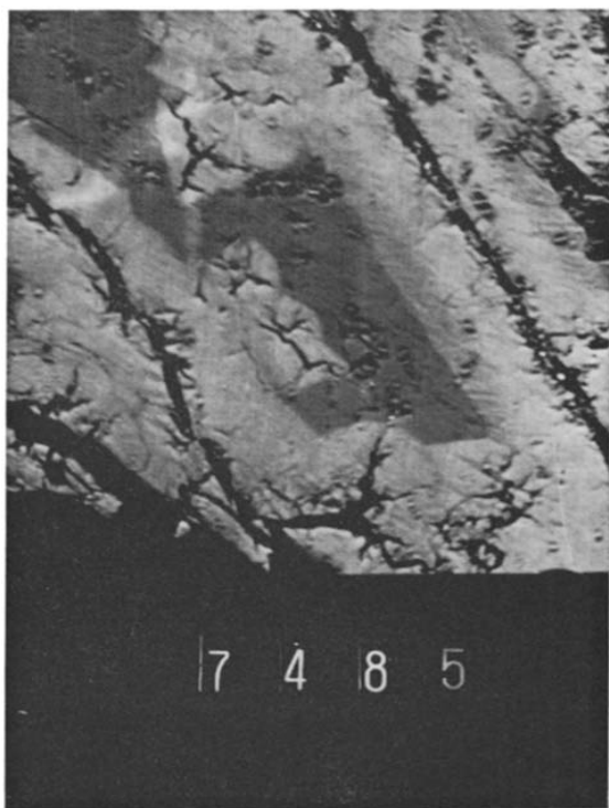
Fig. 5. Electron micrograph of a partly decomposed calcite.
