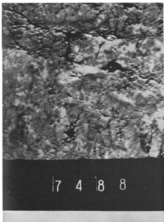
Fig. 6. Electron micrograph of a partly reformed calcite after one decomposition.
