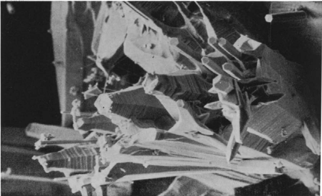
Fig. 12. Sample fracture cross-section after oxidizing at 1223 K. Oxygen flow-rate 300 \text{ Nm}^3 \text{ min}^{-1} . Enlargement 1000 x.
