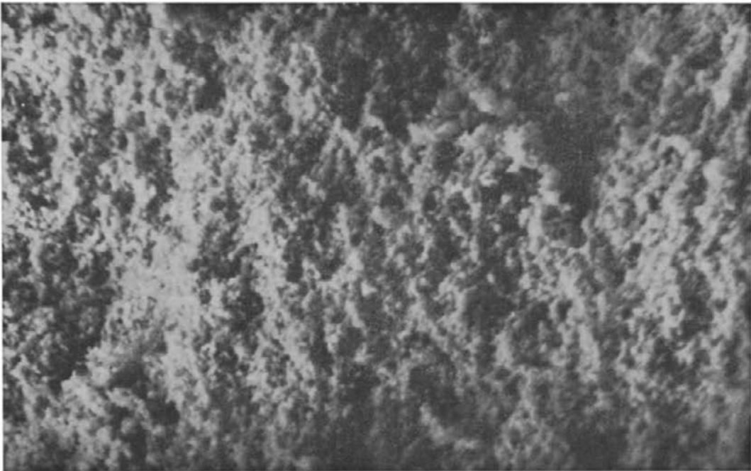
Fig. 2. Cross-section of zinc sulphide with regular structure. Enlargement 3000 x . (simple fracture).
