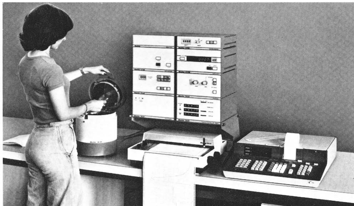
Fig. 1. Mettler TA2000, calorimetric DTA equipment with data transfer system and Hewlett-Packard desk top calculator for automatic evaluation.
