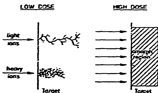
Fig. 26. Schematic drawing of the lattice disorder produced by ion bombardment of high and low doses.
