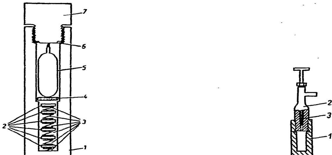
Fig. 13. (a) Steel vessel for kryptonation at high temperature and increased pressure (cf. ref. 108). 1 = Steel vessel body; 2 = sample to be labeled; 3 = metal (Pt) springs; 4 = perforated steel plate; 5 = ampoule containing ^{85}\text{Kr} ; 6 = rubber sealing; 7 = plug screw. (b) Pressure vessel for diffusion kryptonation of melts (cf. ref. 108). 1 = steel jacket; 2 = metal plug; 3 = needle valve.
