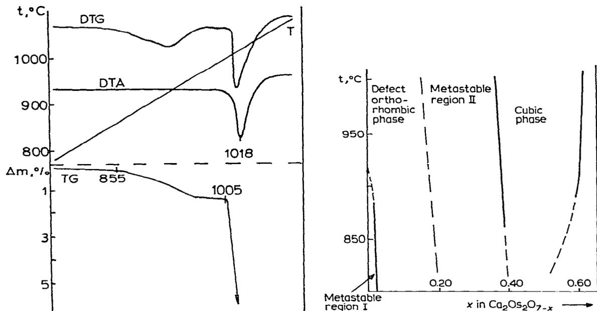
Fig. 1. The thermal decomposition of  $\text{Ca}_2\text{Os}_2\text{O}_7$  in air. Heating rate  $5^\circ\text{C min}^{-1}$ .
