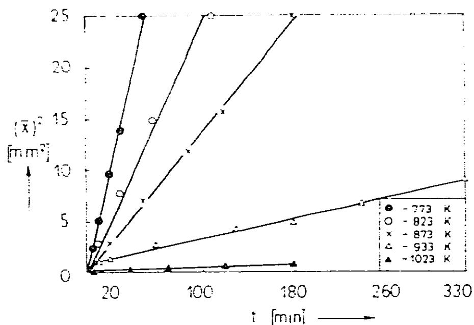
Fig. 5. Linear relationship between the thickness of the layer of oxidation products of galena and the time at the respective temperatures.
