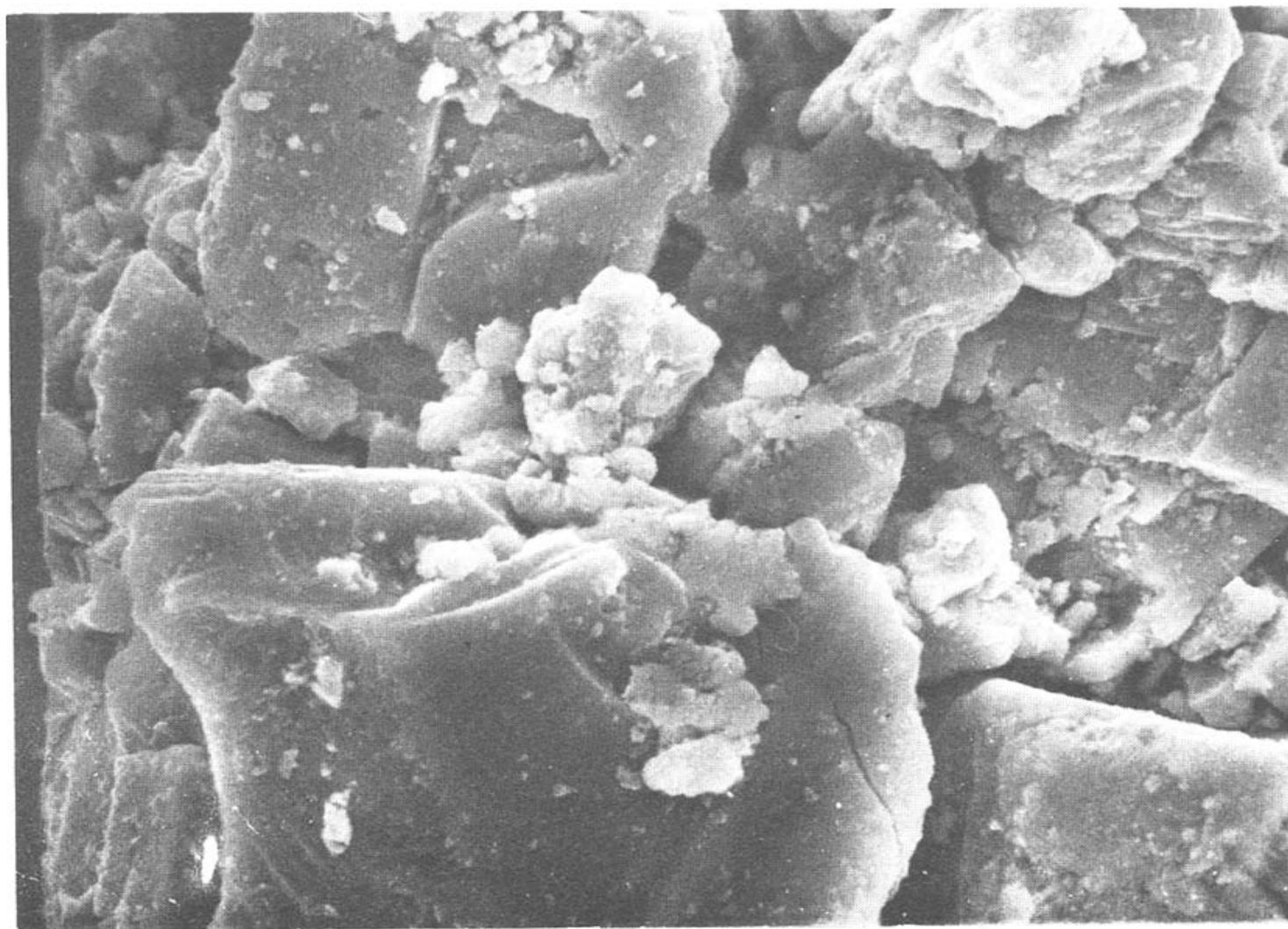
Fig. 7. A fracture of a galena sample under an electron microscope at 3000  $\times$  magnification.
