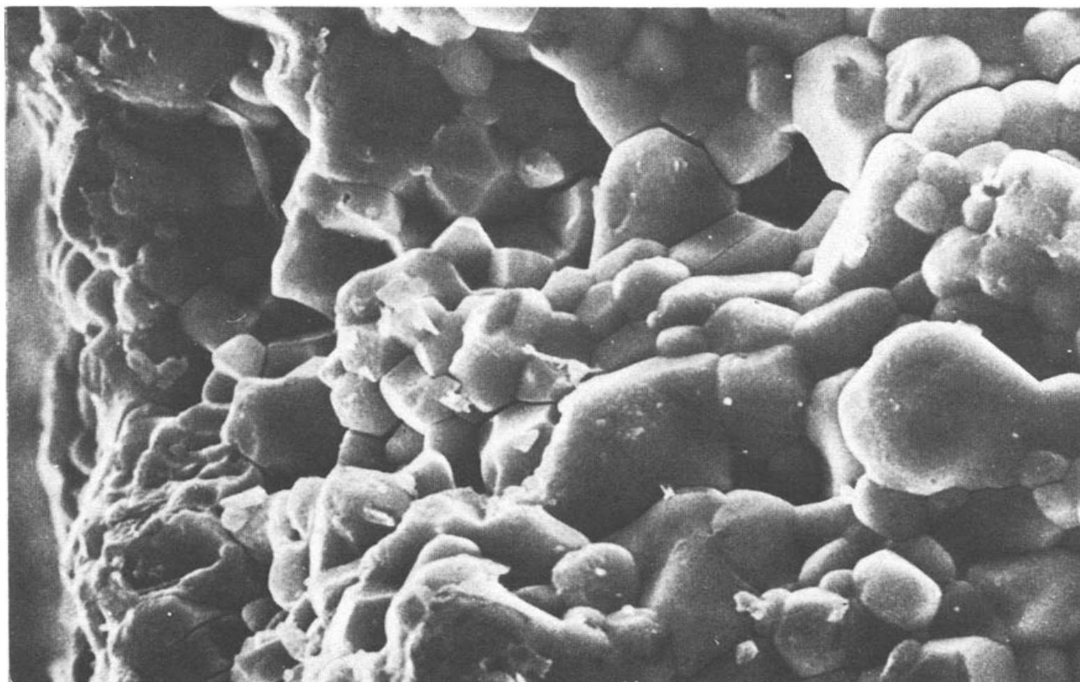
Fig. 10. Structure of s.p. PbS sample oxidized at 1023 K for 150 min. 3000 X magnification.
