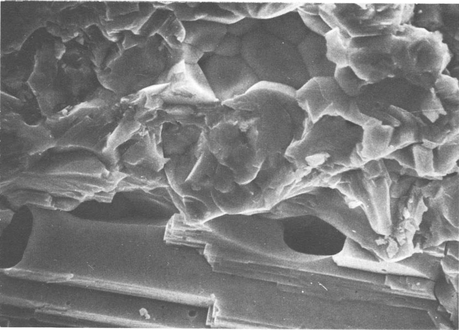
Fig. 8. Structure of the thoroughly reacted layer of galena oxidation products after 150 min at 1023 K. 3000  $\times$  magnification.
