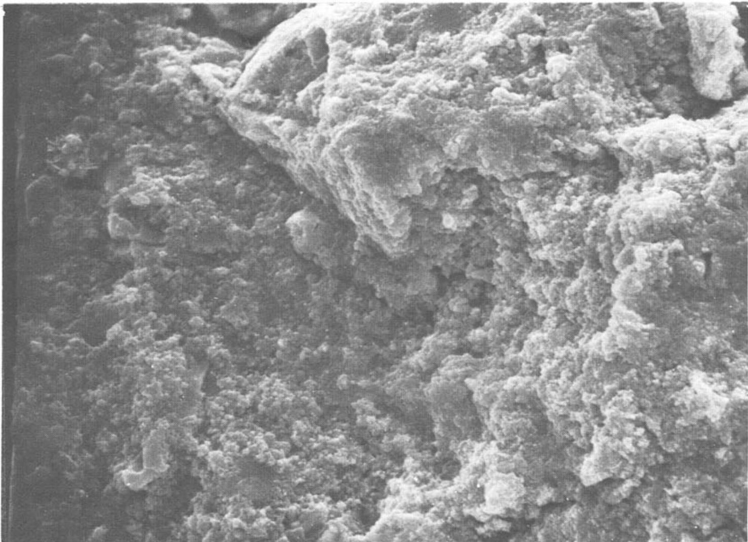
Fig. 9. A fracture of s.p. PbS sample under an electron microscope at 3000  $\times$  magnification.
