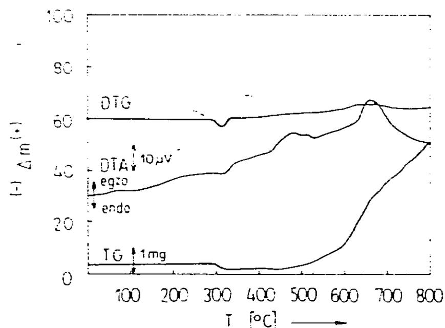
Fig. 1. TG, DTG and DTA curves of galena oxidation in a Mettler thermoanalyser. Heating rate  $4^\circ\text{C min}^{-1}$ .
