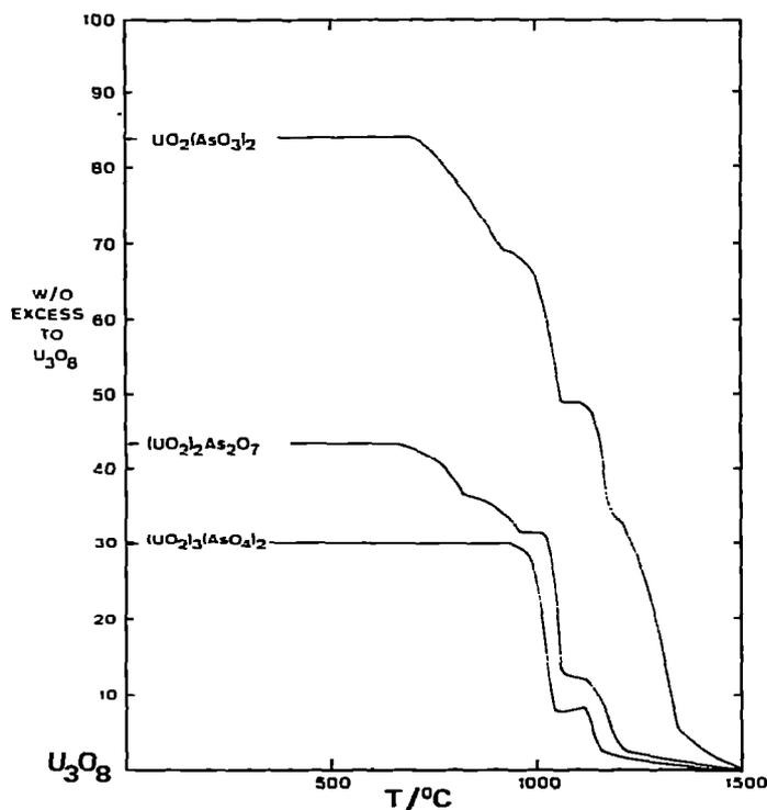
Fig. 2. Thermogravimetric analyses of uranyl arsenates in air ( $2.5^{\circ}\text{C min}^{-1}$ ). Changes of mass are referred to  $\text{U}_3\text{O}_8$ .
