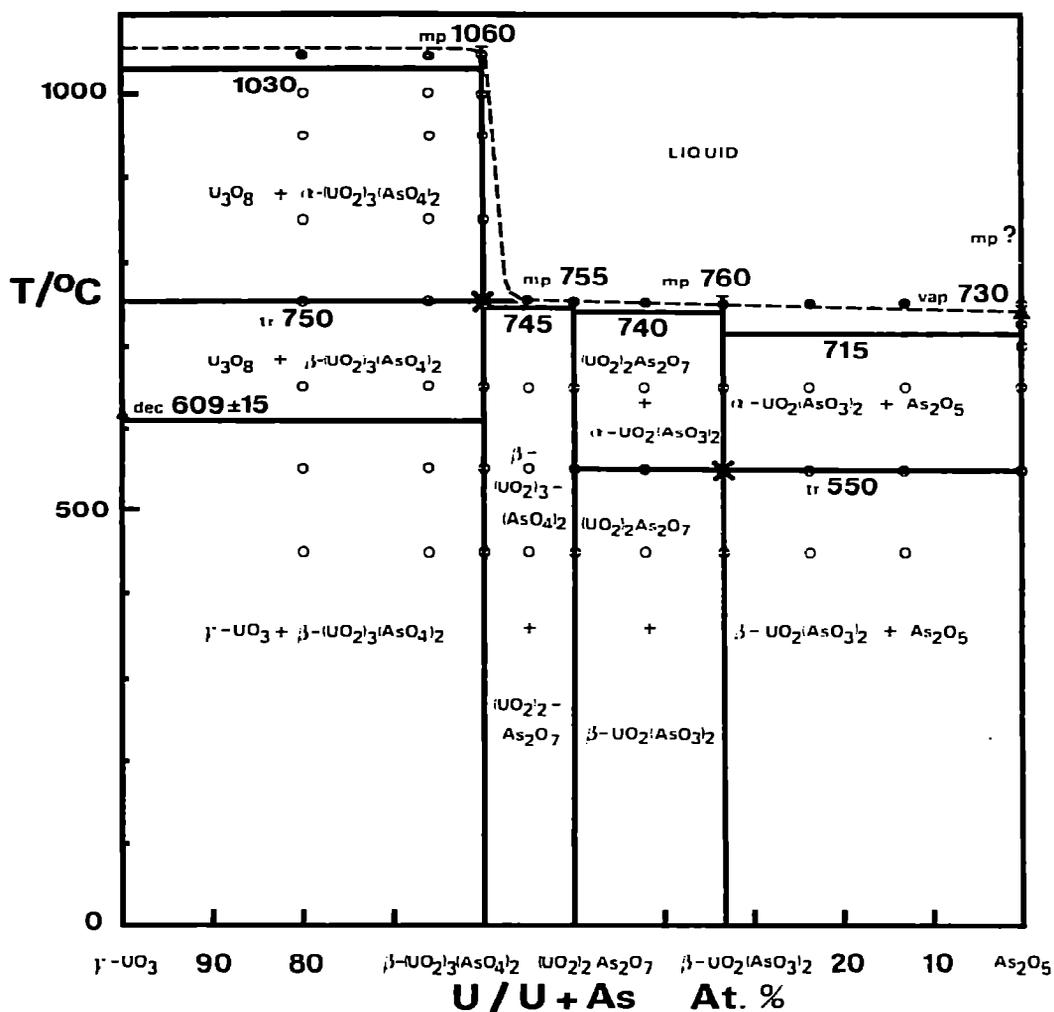
Fig. 3. Tentative subliquidus part of the phase diagram  $\text{UO}_2\text{--As}_2\text{O}_5$  at 0.21 atm oxygen pressure. \* = Phase transitions; --- = maximum accessible temperatures under present conditions;  $\circ$  = isothermal heating;  $\bullet$  = quickly decomposing samples. The accuracy of the temperatures shown is about  $30^\circ\text{C}$ .
