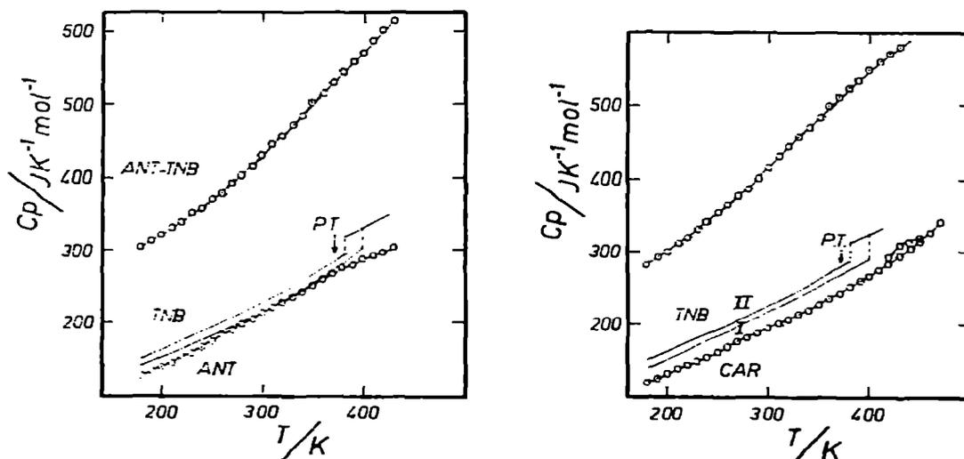
Fig. 5. The temperature dependence of the heat capacity  $C_p$  for anthracene (ANT), 1,3,5-trinitrobenzene (TNB) and the 1 : 1 ANT-TNB complex. Dotted lines designate the quantities:  $C_p$  (TNB I) +  $C_p$  (ANT) and  $C_p$  (TNB II) +  $C_p$  (ANT).
