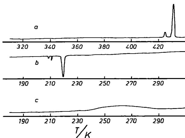
Fig. 3. Thermograms of the 1 : 1 naphthalene—TNB complex recorded at a heating (or cooling) rate of  $2 \text{ K min}^{-1}$ . a, heating from 310 to 410 K; b, cooling from 310 to 180 K (first run); c, heating from 180 to 310 K (for sample after several runs).
