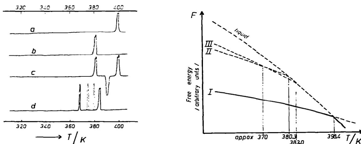
Fig. 1. Selected thermograms of 1,3,5-trinitrobenzene samples recorded at a heating rate of  $2 \text{ K min}^{-1}$ . See the text for explanations.
