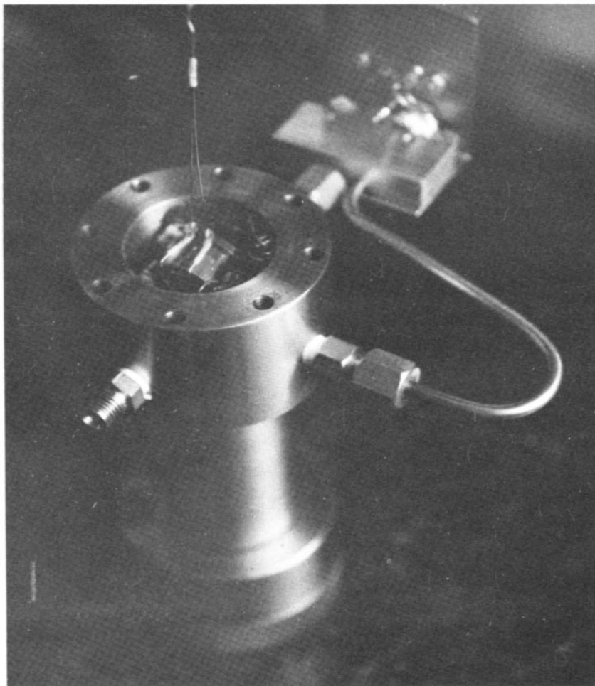
Fig. 5. Photograph of the duPont 951 TGA balance mechanism mounted in the high-pressure enclosure.
