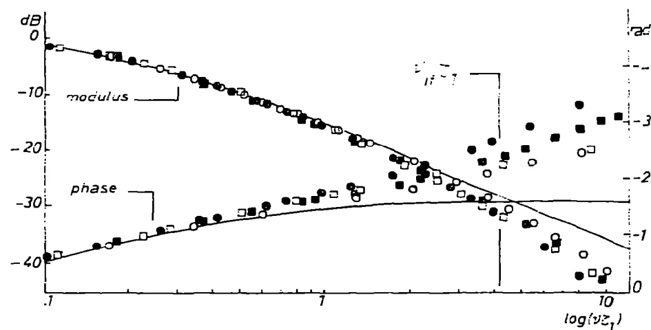
Fig. 2. TF(j\omega) (in Fourier space) for low frequencies corresponding to several high conductivity materials. Modulus (dB) and phase (rad) vs. a reduced scale of frequency [ \log(\nu\tau_1) ]. \square , \circ , \blacksquare , \bullet represent calorimeters A, B, D and F, respectively. The continuous lines represent the modulus and phase of an inverse one-step filter.
