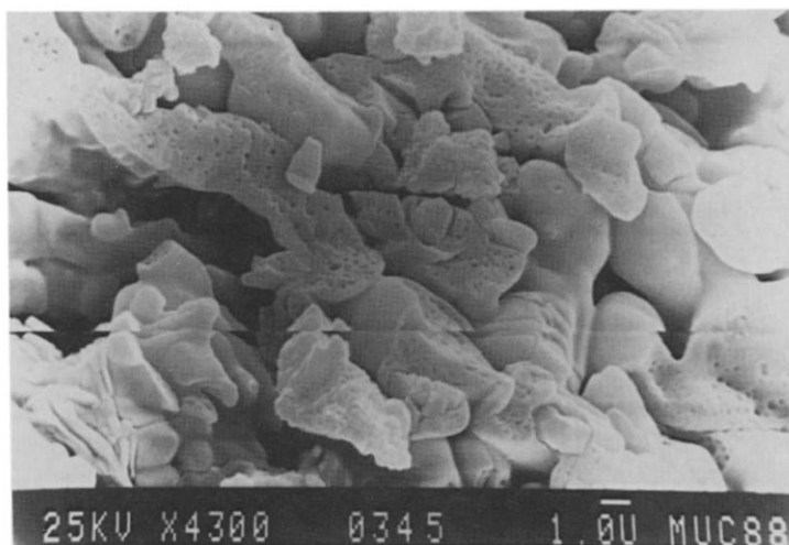
Photograph 3. Scanning electron micrograph of residue from calcination at T = 400^{\circ}\text{C} of (\text{NH}_4)_2\text{Cd}_2(\text{SO}_4)_3 , showing alterations in the morphology of the langbeinite.
