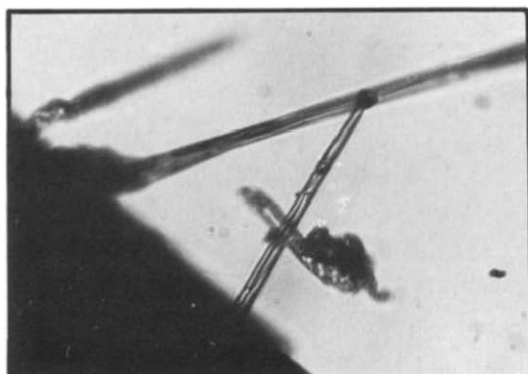
Figs. 7-8. Photographs of the whiskers grown out of the edges of a single crystal of \text{AgN}(\text{SO}_2\text{CH}_3)_2 \cdot 1/4 \text{H}_2\text{O} during the phase transition. The magnifications are 1:100 and 1:250.
