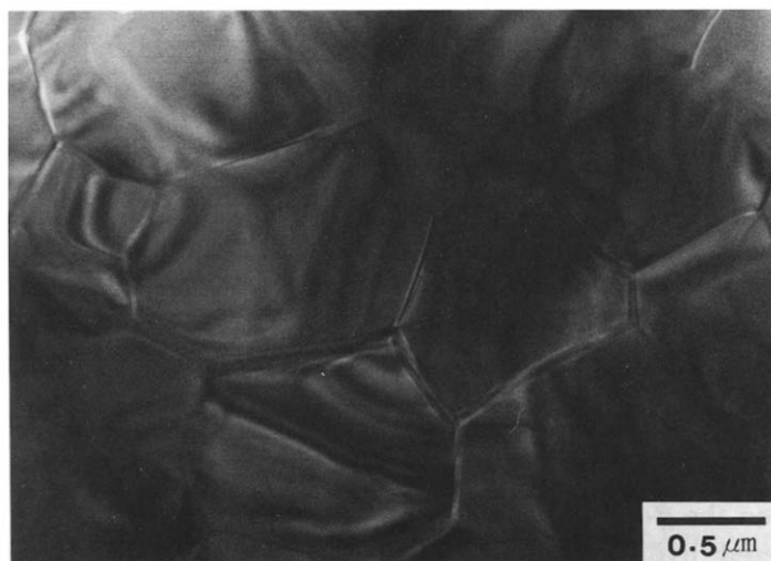
Fig. 8. Transmission electron micrograph of \beta -tricalcium phosphate ceramics sintered at 1150°C.
