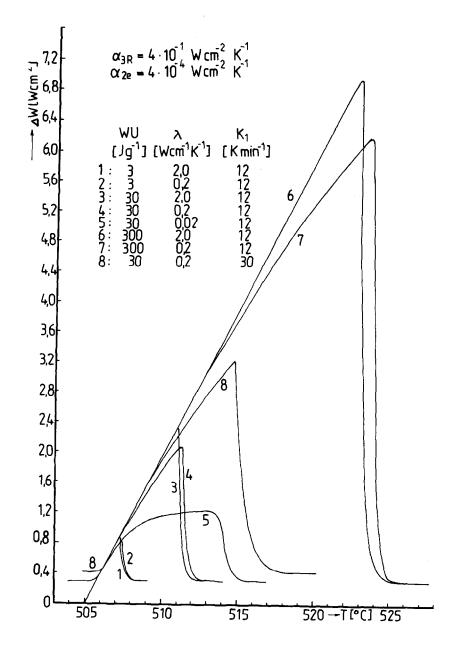
Fig. 5 Numerically calculated transition shapes under different conditions
