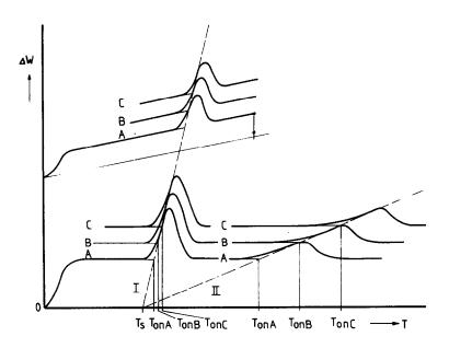
Fig. 6 Relations between true transition temperature, onset temperatures, thermophysical properties, heating rates and heat-transfer coefficients (schematically)
