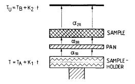
Fig. 1 Calculation model for the influence of the heat-transfer coefficients
