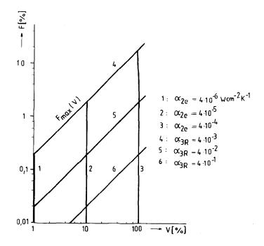
Fig. 4 Deviation F between true and real calorimetrical signal as a function of isothermal distance
