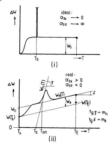
Fig. 3 Graphical representation of mathematical solution The deviation of the real signal  $W_*$  from the ideal signal  $W_s$ is defined as
