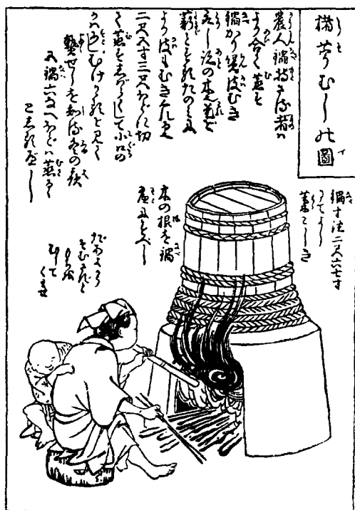
Fig. 34. Boiling of mulberry tree bark strips mixed with ash [17].
