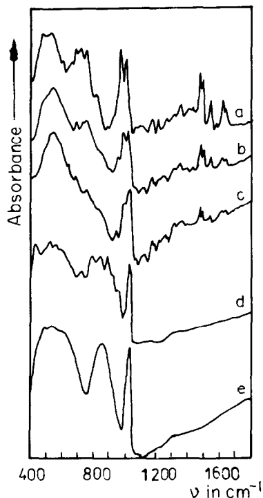
Fig. 3. IR spectra of (\text{PyH})_2\text{V}_6\text{O}_{16} \cdot \text{H}_2\text{O} (a) and of the decomposition products obtained at 275°C (b), 350°C (c), 415°C (d) and 480°C (e).
