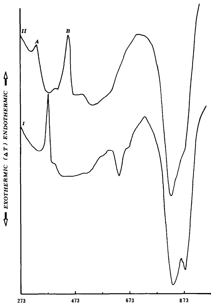
Fig. 5. DTA thermograms (273–973 K) of DMANS (I) and the protonated form (II) showing solid state (A) and solid–liquid (B) phase transitions.
