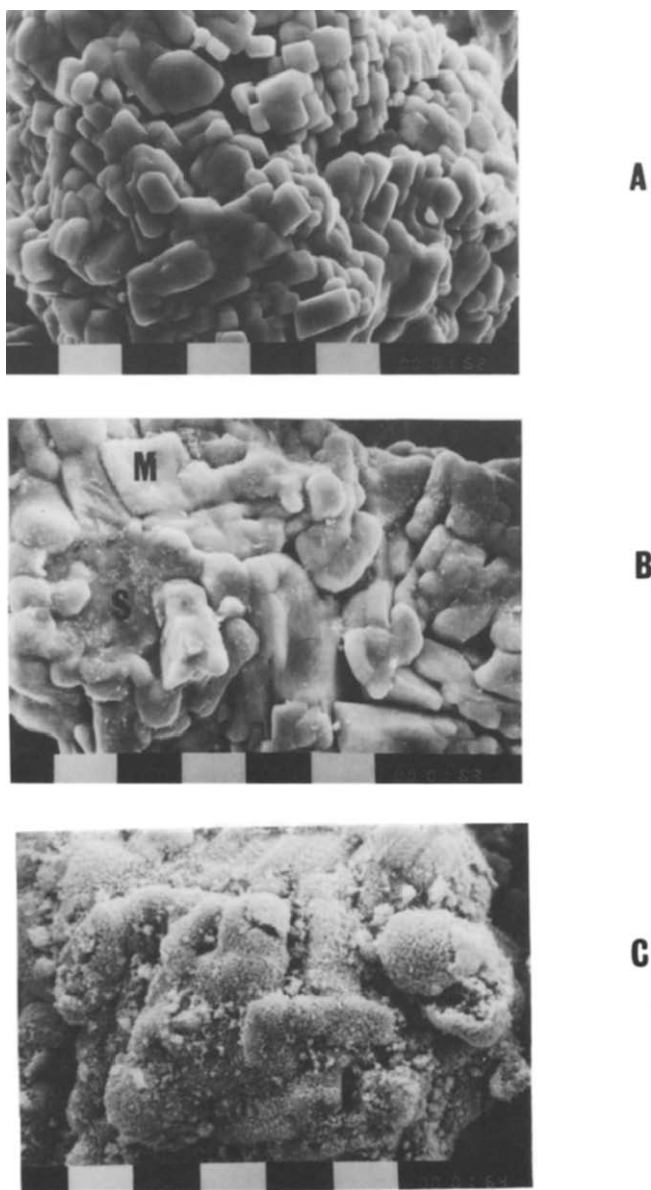
Fig. 3. Scanning electron micrographs (original magnification \times 1620 ; scale bar, 10\ \mu\text{m} ); A, \text{FeVMoO}_7 ; B, \text{FeVMoO}_7 heated at 800^\circ\text{C} ; C, \text{FeVMoO}_7 heated at 1100^\circ\text{C} .
