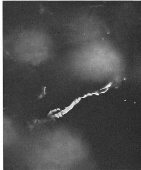
Figs. 14 and 15. The iron filaments formation during the reduction of a magnetite and oxidized magnetite ore with \text{CO-N}_2 mixture at 900^\circ\text{C} . 1200\times .
