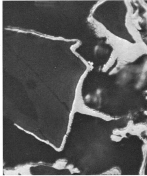
Fig. 12. The formation of an un-uniform iron layer on wustite grains by the reduction of a magnetite ore with \text{CO-N}_2 mixture at 900^\circ\text{C} . 450\times .
