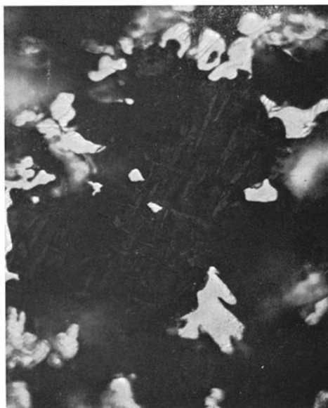
Fig. 10. The formation of an iron layer on certain plains of wustite grains by the reduction of a magnetite ore with CO-N 2 mixture at 900°C. 450 ×.
