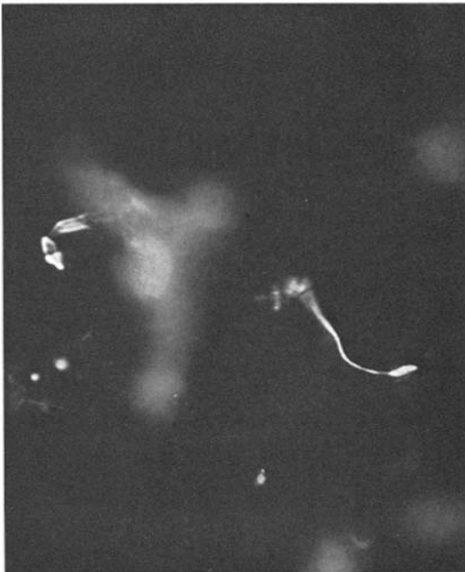
Figs. 14 and 15. The iron filaments formation during the reduction of a magnetite and oxidized magnetite ore with \text{CO-N}_2 mixture at 900^\circ\text{C} . 1200\times .
