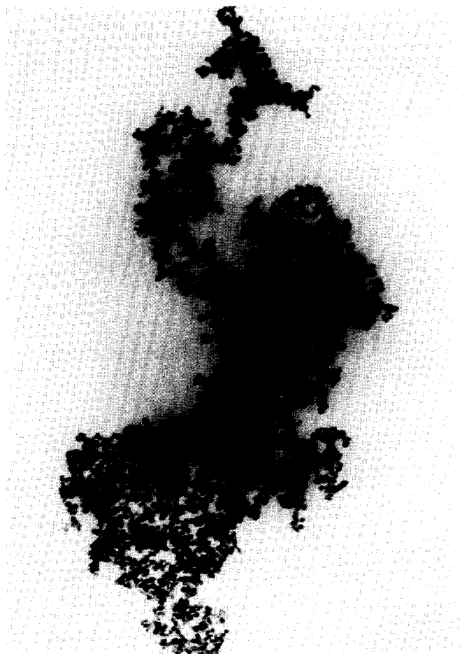
Fig. 4. Electron micrograph of palladium nanoparticles from surnatant of microemulsion at R = 15 (dimension of nanoparticles about 70 \text{ \AA} ).
