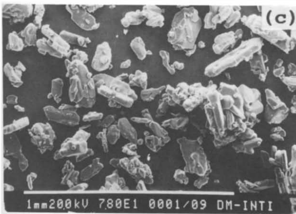
Fig. 1. Electron micrographs of the three samples investigated, as received: (a) Aldrich, (b) Merck, (c) Alfa. Scale: the white horizontal bar represents 10 \mu m in the first case, and 1 mm in the other two cases.
