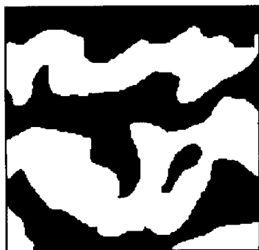
Fig. 2. Schematic representation of microemulsions characterized by a bicontinuous structure. Aqueous microregions (white) and oil microregions (black) are separated by a monolayer of oriented surfactant molecules (for simplicity, the surfactant molecules are not represented).
