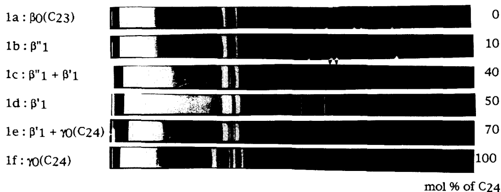
Fig. 1. X-ray diffraction patterns made with a Guinier de Wolff Nonius chamber for C_{23} : C_{24} mixtures when the molar concentration of C_{24} increases at 293 K.
