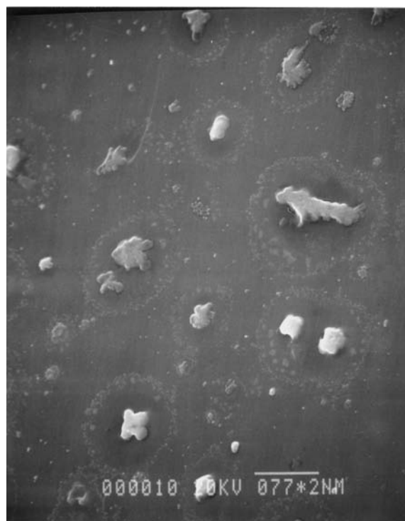
Fig. 12. SEM micrograph of CR10EHMA after 4 h heating at 373 K; detail of Fig. 11.
