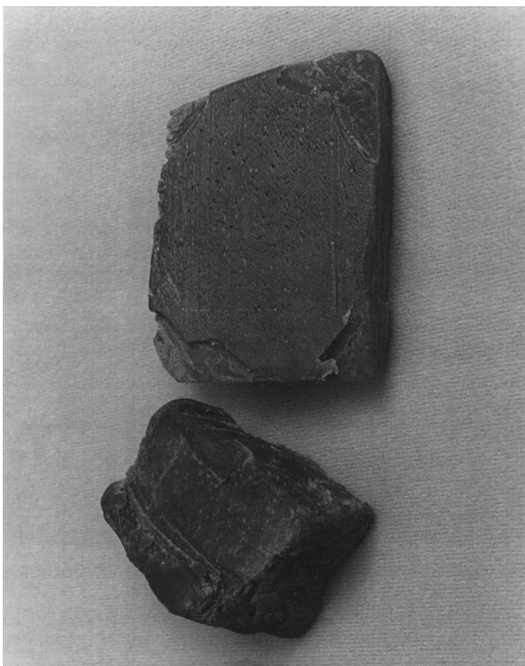
Fig. 1. Block samples of Neoprene FB uncured rubber used in the NASA/MSFC thermal analysis testing: (a) 'new' material kept in cold storage at 40°F for 8 months (left); and (b) 'old' material kept in cold storage for more than 11 years (right).
