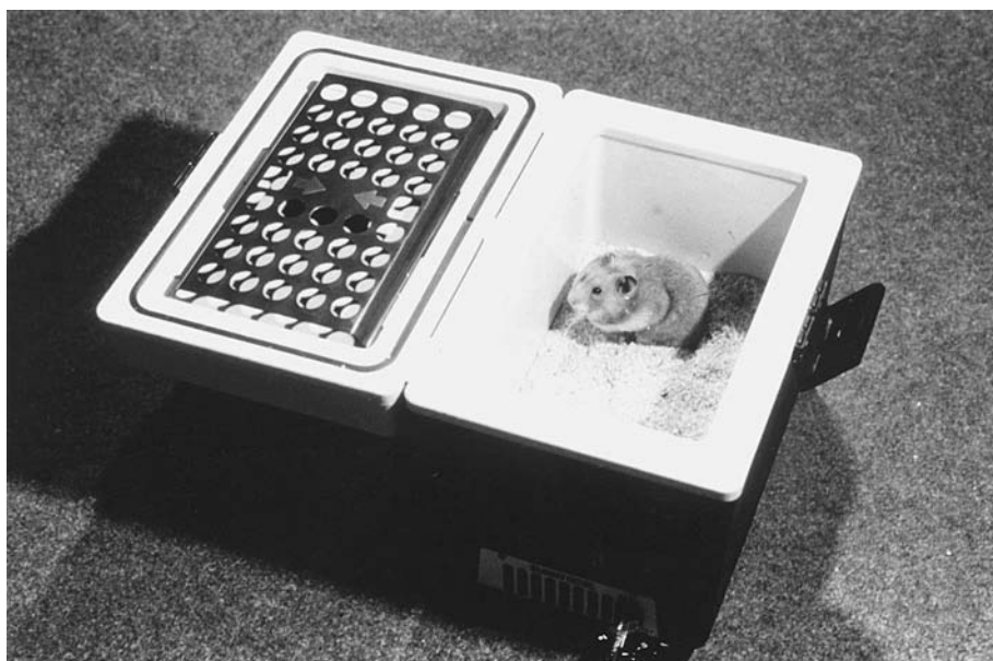
Fig. 3. Golden hamster ( Mesocricetus auratus ) in a camping box calorimeter (PMC) with cover lifted. For further details see text.
