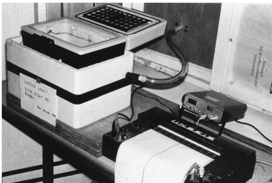
Fig. 1. Camping box calorimeter (PMC) prepared for long term investigations of a bumblebee colony. For better insulation and baseline stability the PMC is placed in a styrofoam box. It is connected to the outside by a longer entrance duct so that the insects have free access to the environment and can forage as usually. One bumblebee passes the right bend of the duct. Two thermocouples for temperature measurements in the box and in the bumblebee nest are visible inside the box.
