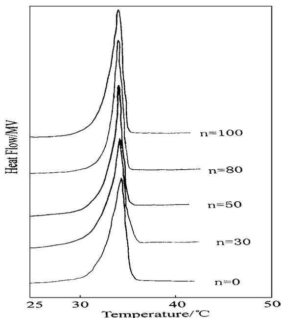
Fig. 2. DSC curves of 22.95% LA-PA binary system after  $n$  cycles.
