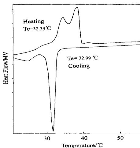
Fig. 1. DSC curve of 43.41% LA–PA binary system in heating–cooling course.
