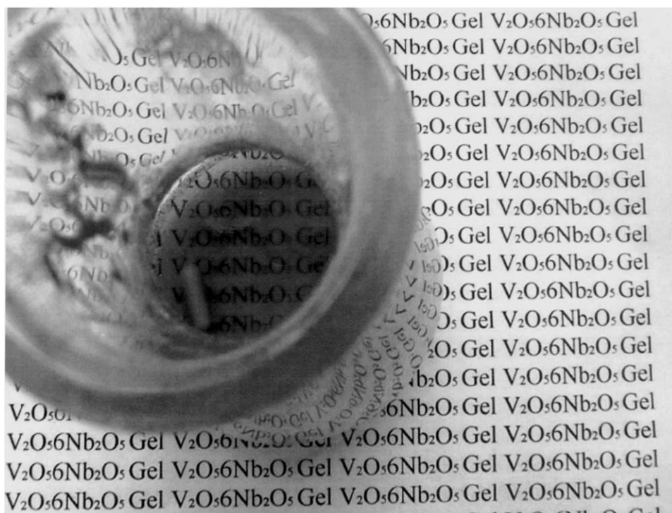
Fig. 2. V-Nb gel dried for 1 day at 50 °C.
