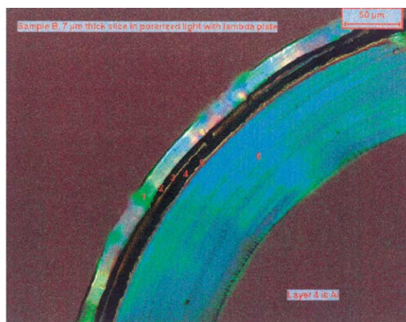
Barrier packaging material #2 (outer surface on the left)
