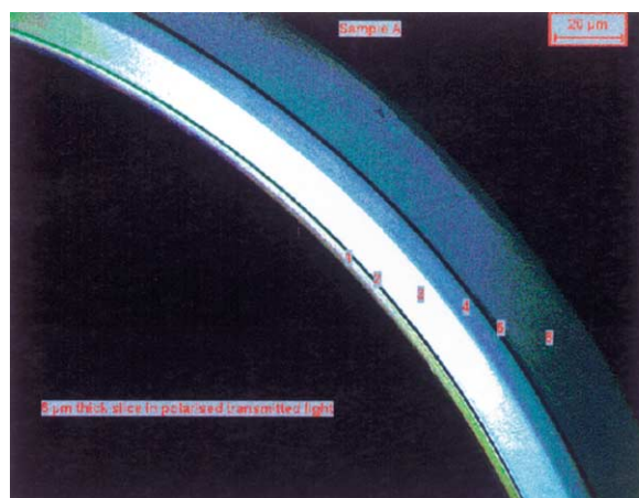
Barrier packaging material #1 (outer surface on the left)
