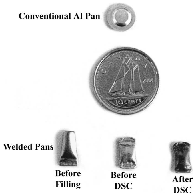
Fig. 1. Comparison between conventional hermetic Al DSC pans and the new stainless steel welded DSC pans. A Canadian 10¢ piece showing the famous “Bluenose” is shown for size comparison.
