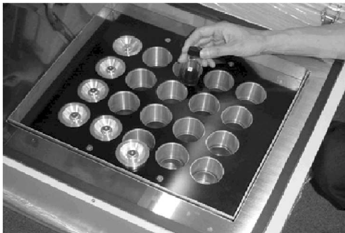
Fig. 1. A 20-channel isothermal microcalorimeter of the heat conduction type. The instrument, based on a design by K. Takahashi, is marketed by Laboratory of Biophysical Chemistry, Kyoto. Glass vessels (50 ml) are placed in thermal contact with thermocouple plates, which are positioned in bores of the heat sink. One of the channels is used as reference.
