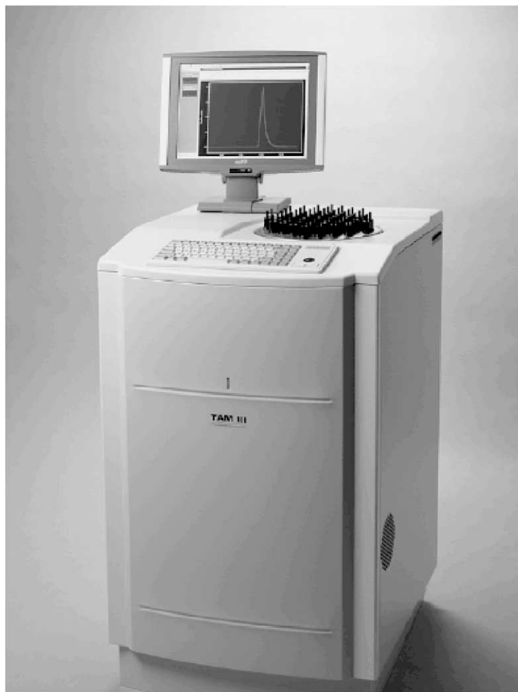
Fig. 3. Thermometric's 48-channel isothermal microcalorimeter. Each channel is a twin heat conduction calorimeter. The two calorimetric units are positioned above one another, with the sample calorimeter at the top and thus accessible for the user. The tubular channels are submerged in a liquid thermostat.
