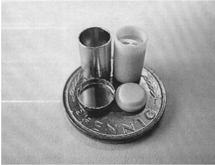
Fig. 4. Crucibles with cover used for DSC measurements; left: platinum, right: \text{Al}_2\text{O}_3 .
