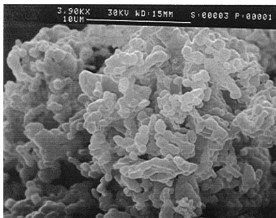
Fig. 14. SEM micrograph of \text{Li}_2\text{CO}_3\text{-Fe}_2(\text{C}_2\text{O}_4)_3\cdot 6\text{H}_2\text{O} mixtures treated under the same experimental conditions adopted in TGA ( x_{\text{Li}} = 0.4028 ). The magnification is reported on the micrograph.
