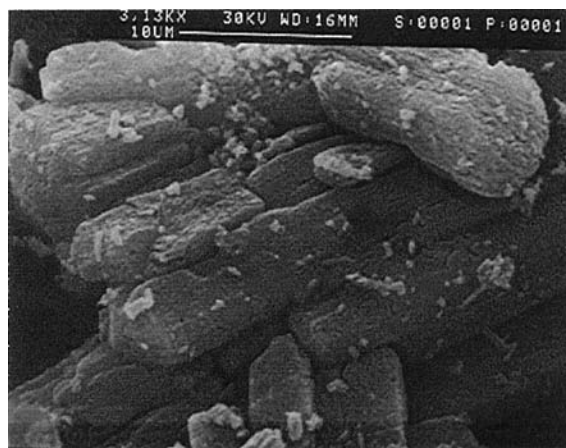
Fig. 4. SEM micrograph of Li 2 CO 3 –FeC 2 O 4 ·2H 2 O mixture treated under the same experimental conditions adopted in TGA ( x_{\text{Li}} = 0.1603 ). The magnification is reported on the micrograph.
