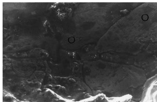
Fig. 5. Scanning electron micrograph of a sample obtained by heating, at a reduced pressure, at 670^\circ\text{C} and then quenched, magnification 2000\times (o-metallic silver).
