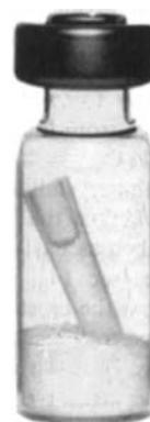
Fig. 2. Sealed glass ampoule containing a sample of powder and a tube with a saturated salt solution (reproduced with permission of Thermometric). The salt solution generates a specific humidity in the air tight ampoule. The heat flow due to any changes in the powder as a consequence of the humidity are recorded.
