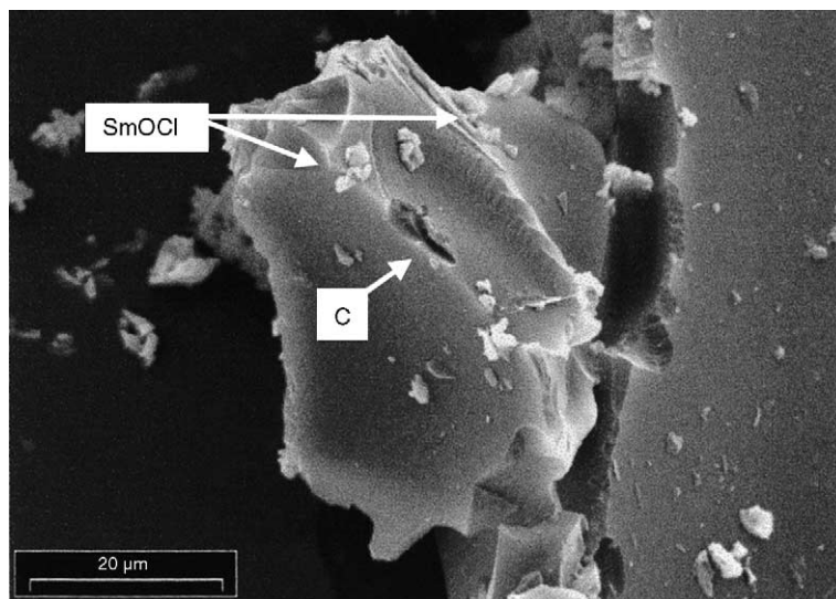
Fig. 4. SEM image of the reaction products at 550 °C. Attacks on carbon surface are observed. Small particles are \text{SmOCl} identified by EDS.
