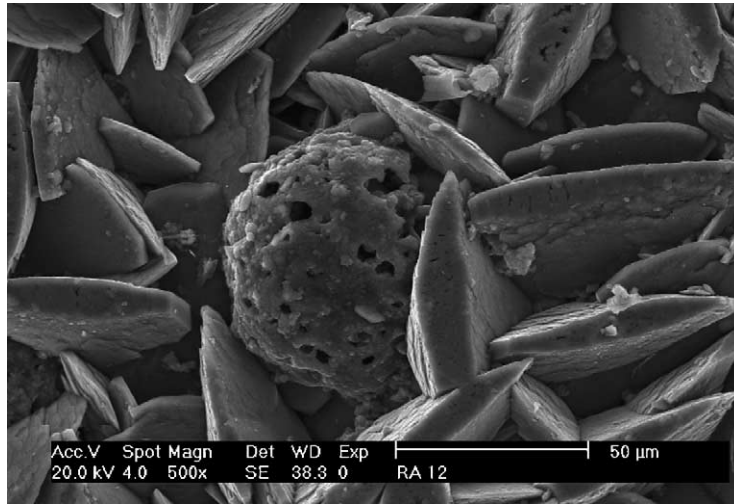
Fig. 3. Scanning electron micrograph of a damage layer showing gypsum crystals with lamellar habit which embed a spongy carbonaceous particle.
